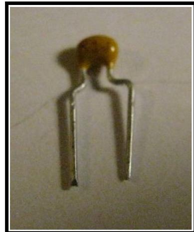
Install the 150pf cap between the two PN2222 transistor locations and then solder in the two 100pf caps just above the 2 lay down 10K resistors. Your 100pf caps might look a little different as they may be NPO ceramic disc caps....
